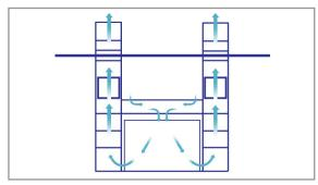
Side Downdraft booths intake air from the cleaner upper levels of the shop through a filtered booth ceiling. The filtered air is drawn down and away from the product through exhaust filters at the floor level, along both sides.
