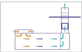
Modified Downdraft booths intake fresh air from the cleaner upper levels of the shop through a filter bank located in the booth ceiling, near the product doors. The filtered air is drawn down through the booth to an exhaust filter system at the opposite end.
