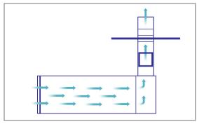
Crossdraft booths intake air through filters in the product doors. The clean, filtered air is drawn through the booth and exhausted through a filter system at the opposite end.
