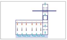
Downdraft booths take in fresh air from the cleaner upper levels of the shop through a filtered booth ceiling. The filtered air is drawn down and away from the product into the filtered exhaust pit located in the floor.
