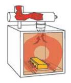
prevents distortion of the part during the process. The primary and secondary water suppression system along with the monitoring of both the oven and afterburner chamber temperatures ensures a safe controlled burn-off.
